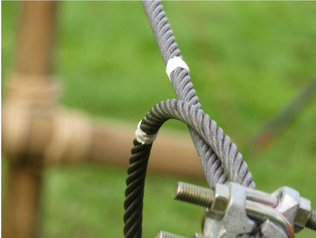
Figure 58 Hawser Slippage Inspection
