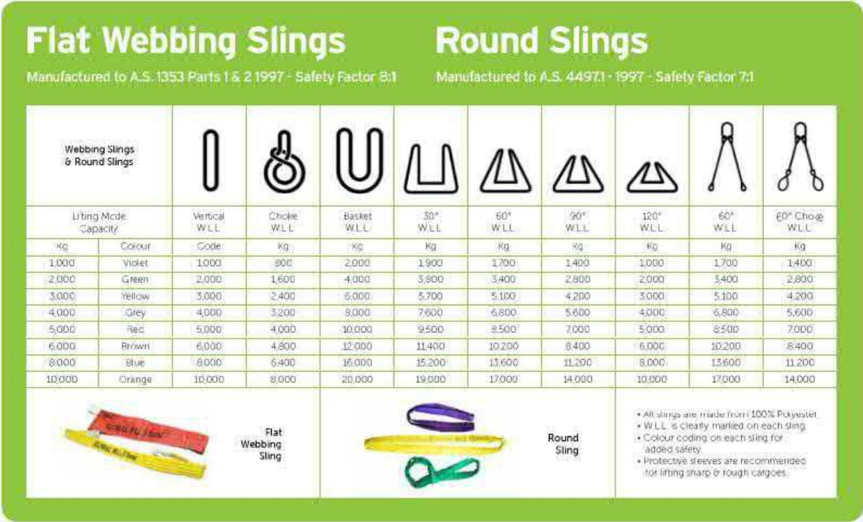
Figure 10 Flat Webbing & Round Sling Working Load Limit (EnergySafe Victoria for slings manufactured to AS1353.1, AS1353.2 and AS4497.1)
